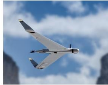
Orbiter 2b Aeronautics ca. 10 kg ca. 3 / 1.5 m / 0.4 m 33 – 50 kts (60-90 km/hm)
